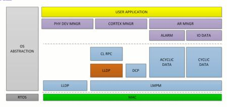
The Profinet IO Device-side Protocol Stack consists of hardware independent and hardware dependent components. These components communicate via message queues. The hardware dependent part consists of the interface for the Ethernet MAC controller and timer functions.
